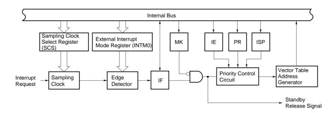
Figure 18-1. Basic Configuration of Interrupt Function (2/2)
