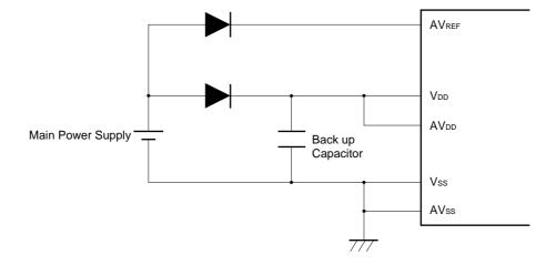
Figure 14-11. AVDD Pin Connection
