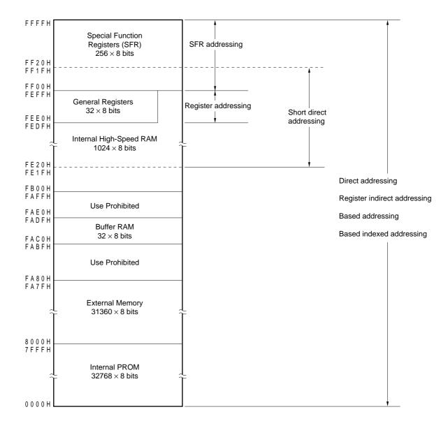
Figure 5-16. Data Memory Addressing ( $\mu$ PD78P014, 78P014Y)
