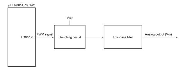
Figure 8-13 shows an example in which PWM output is converted to an analog voltage and used in a voltage synthesizer type TV tuner.
