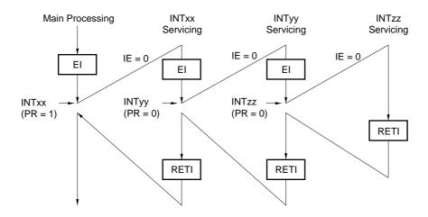
During interrupt INTxx servicing, two interrupt requests, INTyy and INTzz are acknowledged, and a multiple interrupt is generated. An EI instruction is issued before each interrupt request acknowledge, and the interrupt request acknowledge enable state is set.
