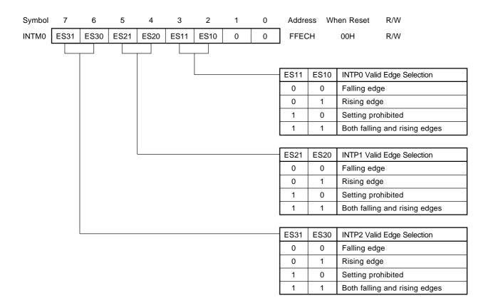
Caution Set the valid edge for INTP0/TI0/P00 after setting bits 1 through 3 (TMC01 to TMC03) of 16-bit timer mode control register to 000 to stop the timer operation.
