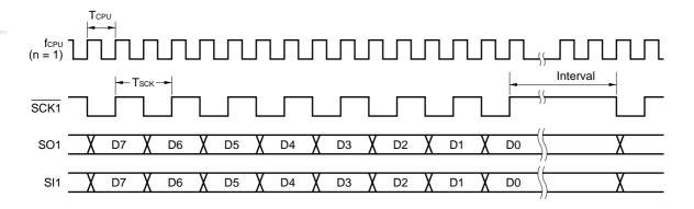
fcpu : CPU clock (set by bit 0 to bit 2 (PCC0 to PCC2) of processor clock control register (PCC))
