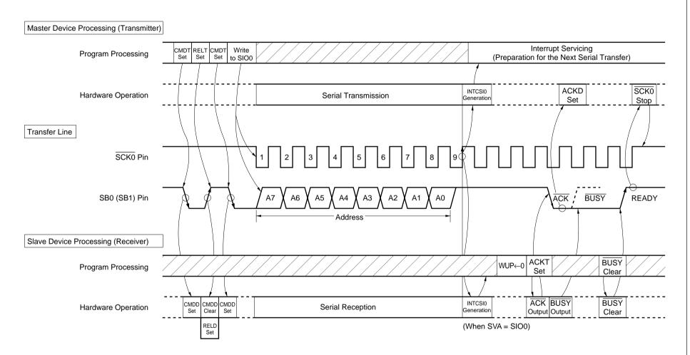
Figure 16-30. Command Transmission from Master Device to Slave Device
