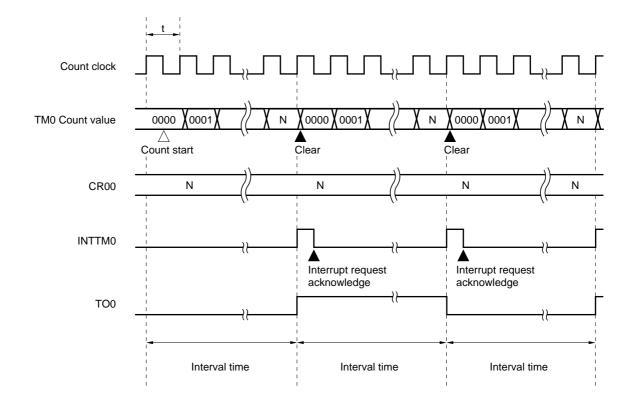
Figure 8-11. Interval Timer Operation Timings
