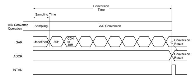
Figure 14-4. A/D Converter Basic Operation
