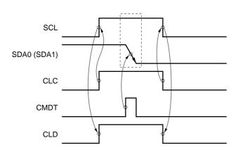
Figure 16-47. Start Condition Output
