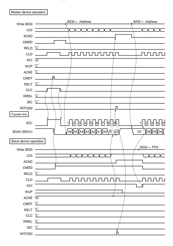
Figure 16-45. Data Transmission from Master to Slave (Both Master and Slave Selected 9-Clock Wait) (2/3)
