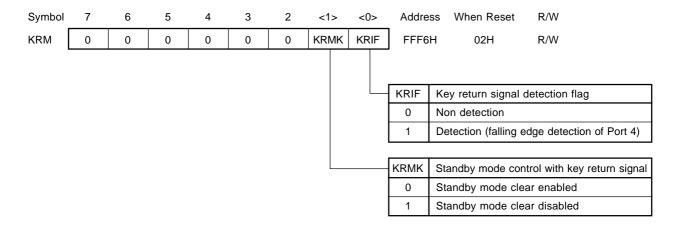
Caution When falling edge detection is used in Port 4, take care to clear KRIF to 0 (KRIF is not automatically cleared to 0).
