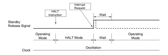
**Remarks** 1. The broken line indicates the case when the interrupt request which has cleared the standby status is acknowledged.
