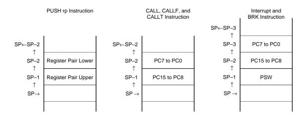
Figure 5-10. Data to be Reset from Stack Memory
