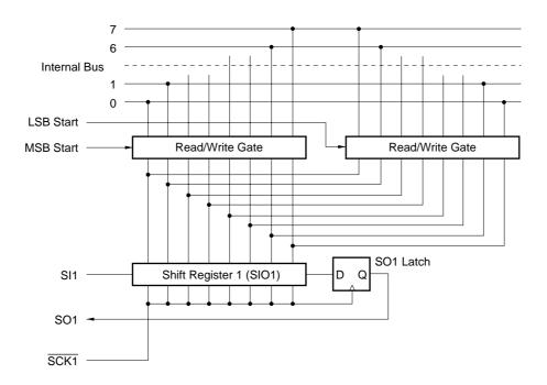
Figure 17-6. Circuit of Switching in Transfer Bit Order
