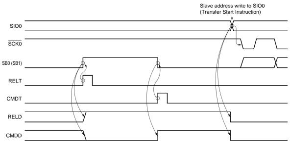
Figure 16-22. RELT, CMDT, RELD and CMDD Operations (Master)
