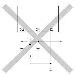
**Remark** When using a subsystem clock, replace X1 and X2 with XT1 and XT2, respectively. Further, insert resistors in series on the side of XT2.
