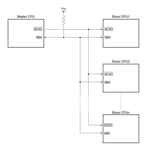
Figure 15-1. Serial Bus Interface (SBI) System Configuration Example
