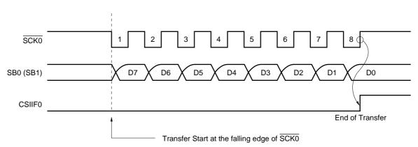
Figure 15-33. 2-Wire Serial I/O Mode Timings
