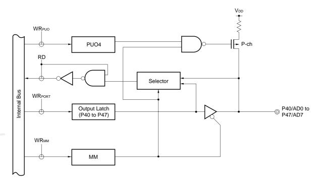
Figure 6-11. P40 to P47 Block Diagrams
