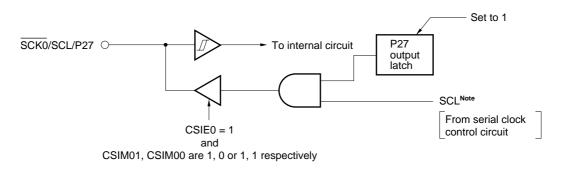
**Note** Level of SCL signal is determined by the following logic in the Figure 16-52.
