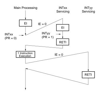
The interrupt request INTyy generated during interrupt INTxx servicing is not acknowledged because the interrupt priority is lower than that of INTxx, and a multiple interrupt is not generated. INTyy request is retained and acknowledged after execution of 1 instruction execution of the main processing.
