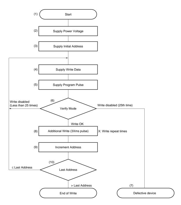
Figure 22-3. Write Procedure Flowchart
