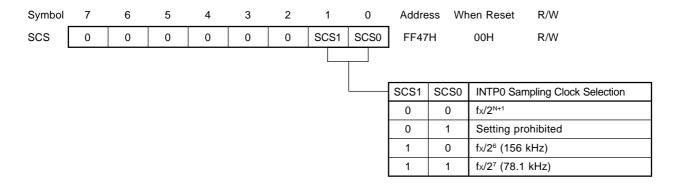
Caution  $fx/2^{N+1}$  is a clock to be supplied to the CPU and  $fx/2^6$  and  $fx/2^7$  are clocks to be supplied to the peripheral hardware.  $fx/2^{N+1}$  stops in the HALT mode.
