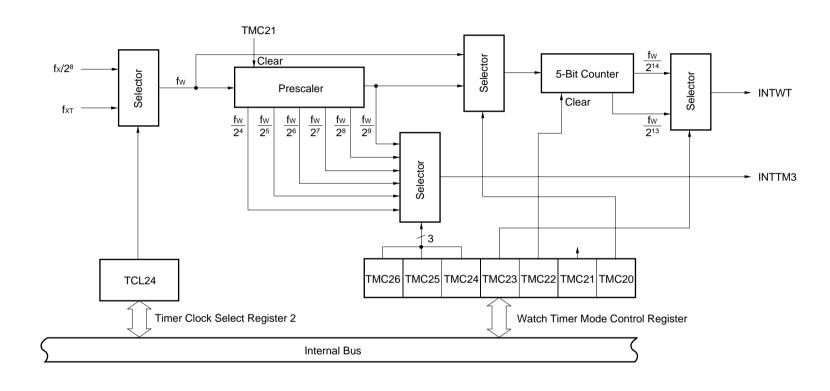
Figure 10-1. Watch Timer Block Diagram
