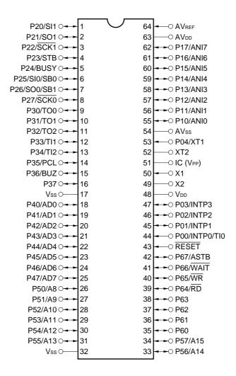
Cautions 1. Connect IC (Internally Connected) pin directly to Vss.
