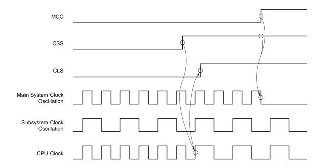
Figure 7-7. Main System Clock Stop Function (2/2)
