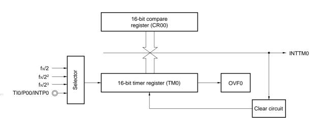
Figure 8-10. Interval Timer Configuration Diagram
