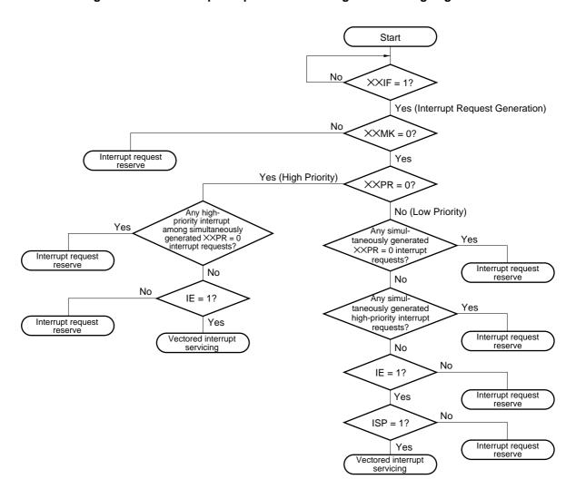
Figure 18-12. Interrupt Request Acknowledge Processing Algorithm
