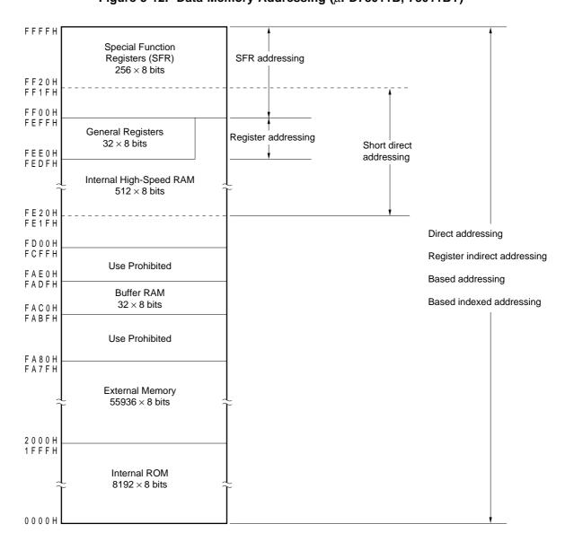
Figure 5-12. Data Memory Addressing ( $\mu$ PD78011B, 78011BY)
