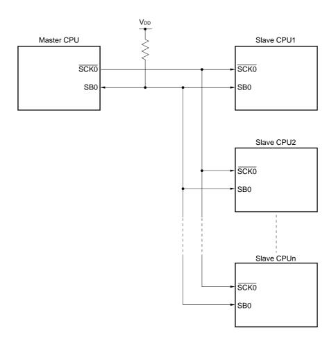
Figure 16-1. Serial Bus Interface (SBI) System Configuration Example
