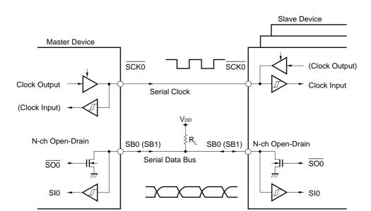
Figure 15-27. Pin Configuration
