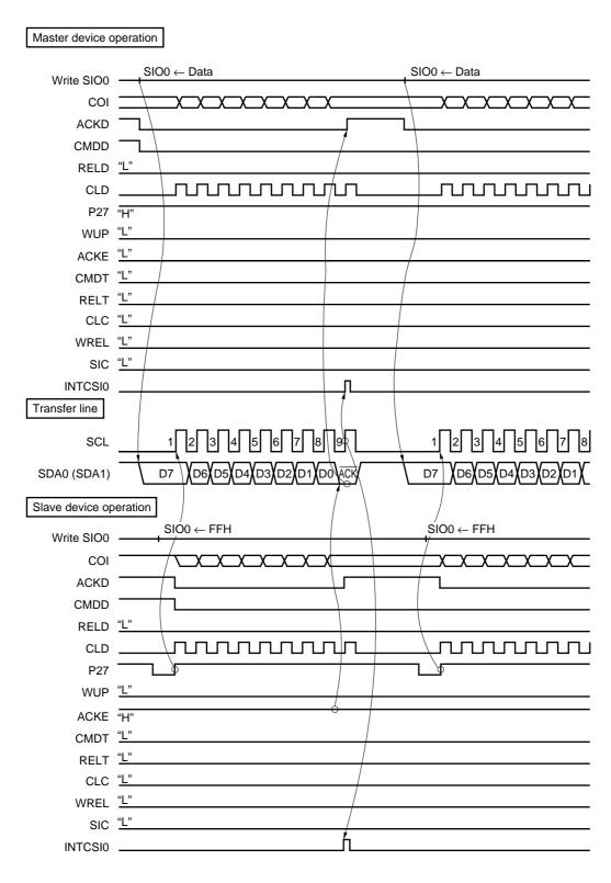
Figure 16-45. Data Transmission from Master to Slave (Both Master and Slave Selected 9-Clock Wait) (3/3)
