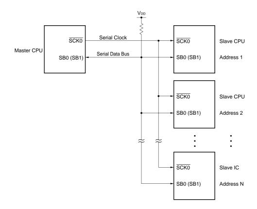
Figure 16-12. Example of Serial Bus Configuration with SBI
