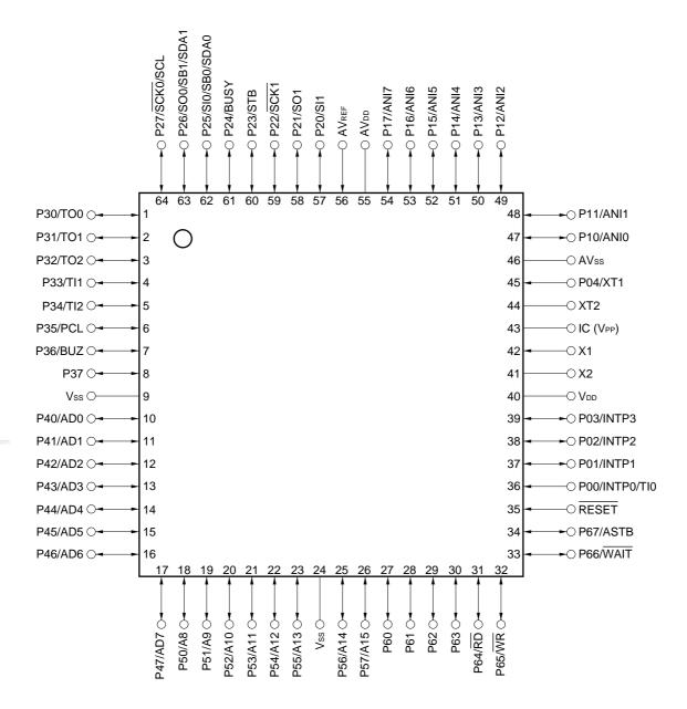
Cautions 1. Connect IC (Internally Connected) pin directly to Vss.
