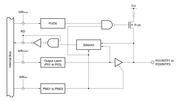
Figure 6-3. P01 to P03 Block Diagrams
