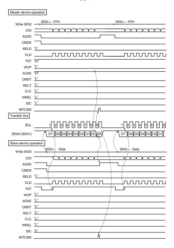
Figure 16-46. Data Transmission from Slave to Master (Both Master and Slave Selected 9-Clock Wait) (3/3)
