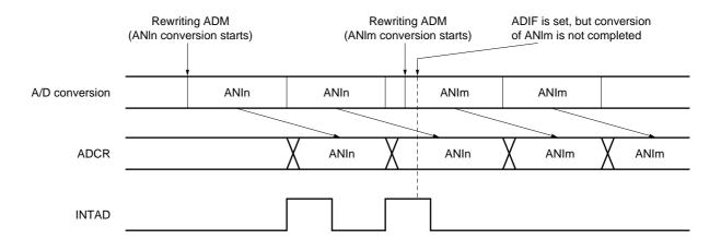
Figure 14-10. A/D Conversion End Interrupt Request Generation Timing
