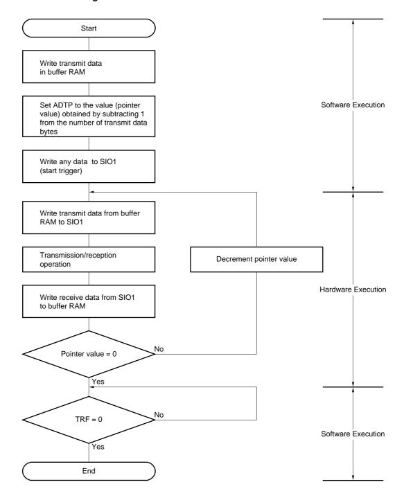
Figure 17-8. Basic Transmit/Receive Mode Flowchart
