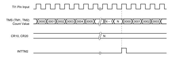
Caution Even if the 16-bit timer/event counter mode is used, when the TM1 count value matches the CR10 value, interrupt request (INTTM1) is generated and the F/F of 8-bit timer/event counter output control circuit 1 is inverted. Thus, when using 8-bit timer/event counter as 16-bit interval timer, set the mask flag TMMK1 to 1 to disable INTTM1 acknowledgment.
