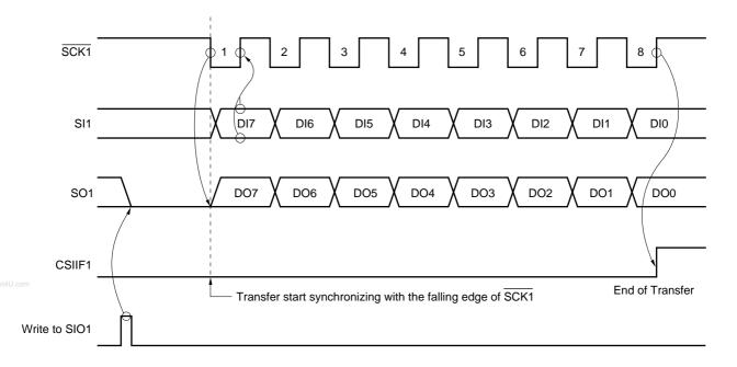
Figure 17-5. 3-Wire Serial I/O Mode Timings
