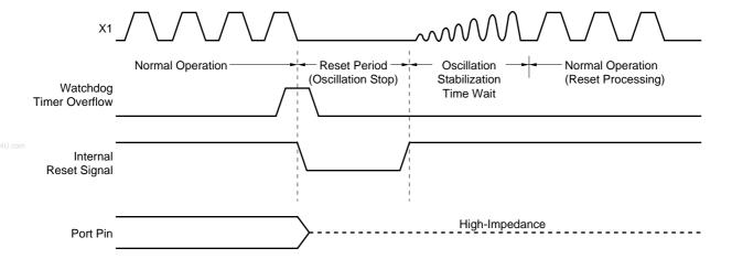
Figure 21-4. Timing of Reset in STOP Mode by RESET Input
