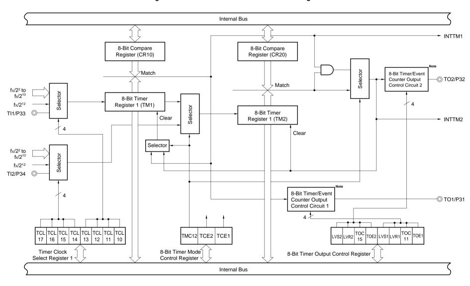
Figure 9-1. 8-Bit Timer/Event Counter Block Diagram
