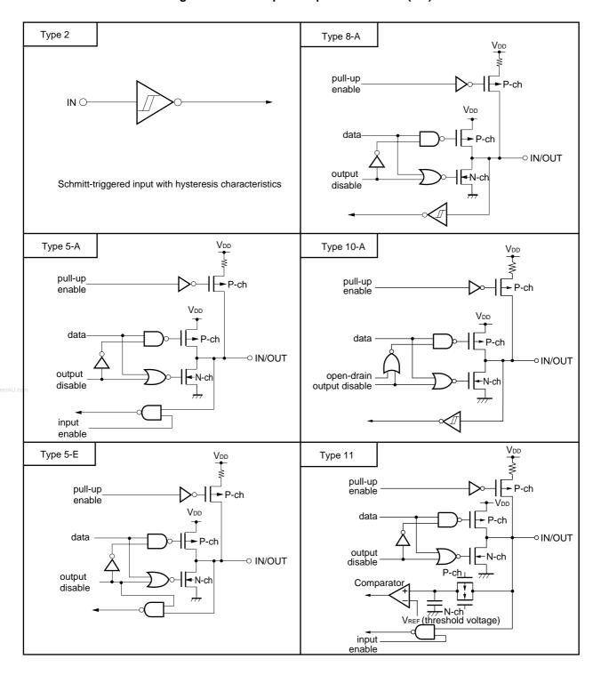
Figure 3-1. Pin Input/Output Circuit List (1/2)
