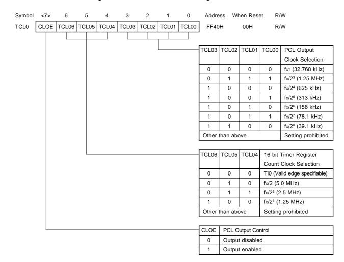
Figure 8-4. Timer Clock Select Register 0 Format
