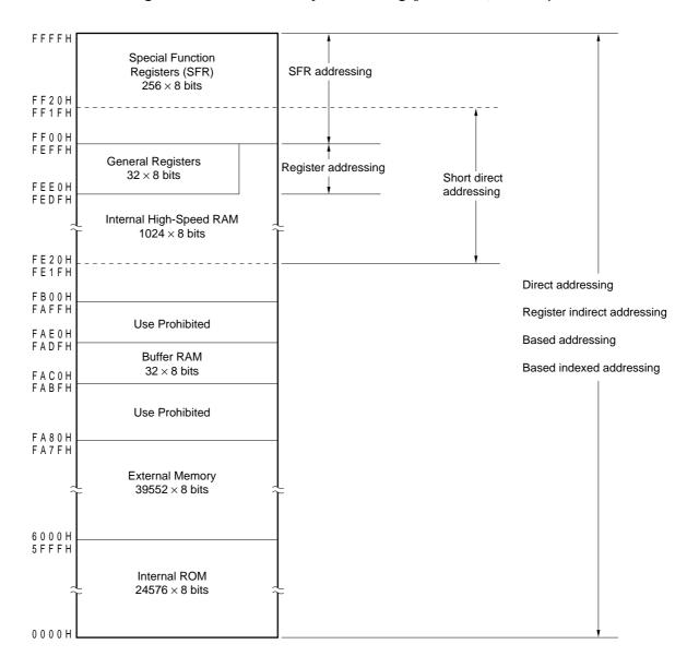
Figure 5-14. Data Memory Addressing ( $\mu$ PD78013, 78013Y)
