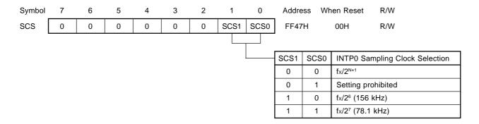
Caution  $f_x/2^{N+1}$  is the clock supplied to the CPU, and  $f_x/2^6$  and  $f_x/2^7$  are clocks supplied to peripheral hardware.  $f_x/2^{N+1}$  is stopped in HALT mode.
