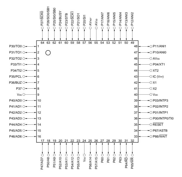
Cautions 1. Connect IC (Internally Connected) pin directly to Vss.
