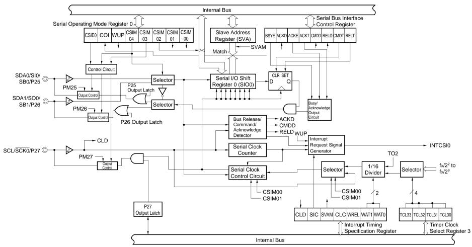
Remark Output Control performs selection between CMOS output and N-ch open-drain output.
