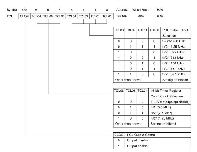
Figure 12-3. Timer Clock Select Register 0 Format
