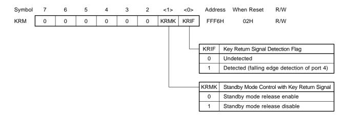
Caution When falling edge detection is used in port 4, be sure to clear KRIF to 0 (KRIF cannot be cleared to 0 automatically).
