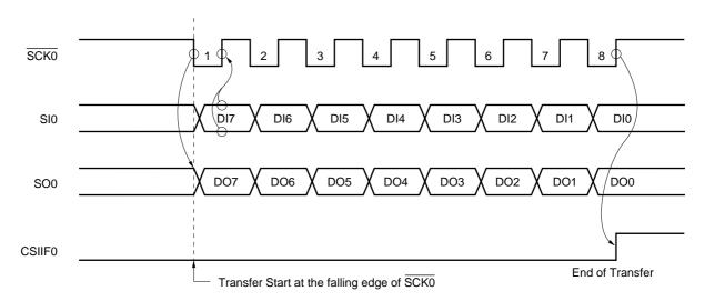
Figure 15-8. 3-Wire Serial I/O Mode Timings
