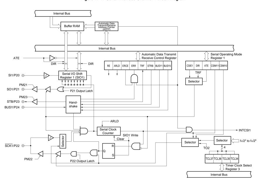
Figure 17-1. Serial Interface Channel 1 Block Diagram
