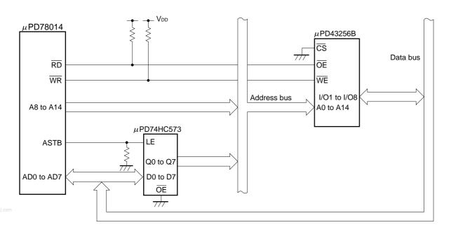
Figure 19-7. Example of Memory Connection with  $\mu$ PD78014
