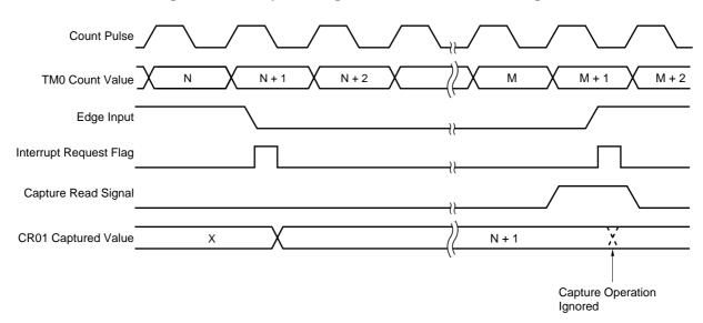
Figure 8-22. Capture Register Data Retention Timings
