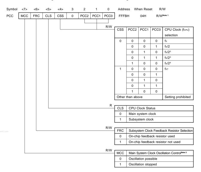
Figure 7-3. Processor Clock Control Register Format
