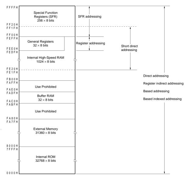
Figure 5-15. Data Memory Addressing ( $\mu$ PD78014, 78014Y)
