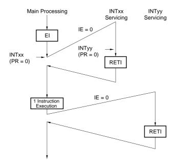
Because interrupts are not enabled in interrupt INTxx servicing (an EI instruction is not issued), interrupt request INTyy is not acknowledged, and a multiple interrupt is not generated. The INTyy request is reserved and acknowledged after 1 instruction execution of the main processing.
