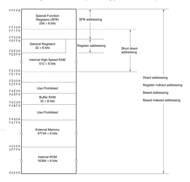
Figure 5-13. Data Memory Addressing ( $\mu$ PD78012B, 78012BY)
