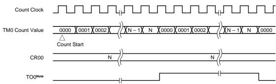
**Note** Initial value of TO0 output can be set at bits 2 and 3 (LVR0 and LVS0) of the 16-bit timer output control register (TOC0).
