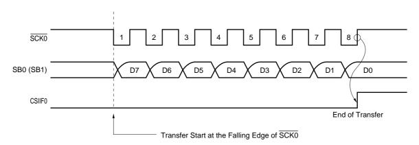
Figure 16-34. 2-Wire Serial I/O Mode Timings
