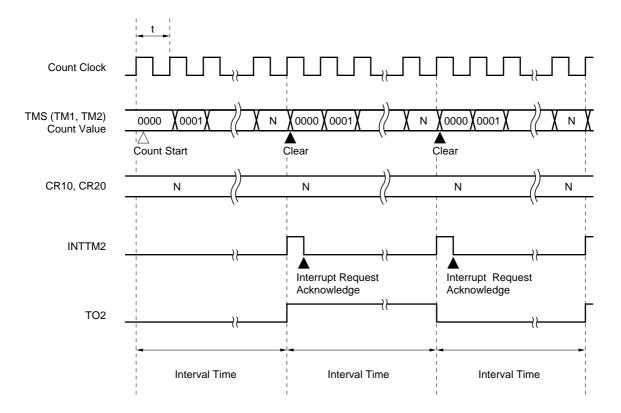
Figure 9-11. Interval Timer Operation Timings
