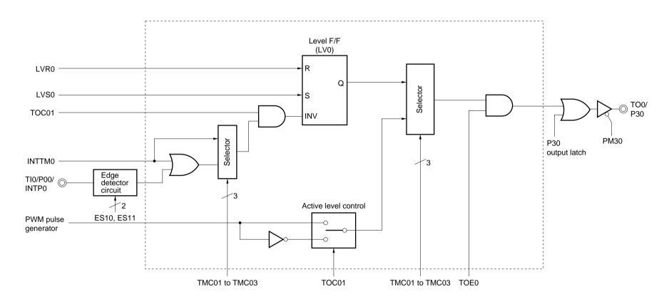
**Remark** The circuitry enclosed by the dotted line is the output control circuit.
