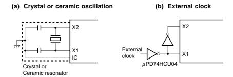
Caution The STOP mode cannot be set while an external clock is being input. This is because the X1 pin is short-circuited to Vss in the STOP mode.
