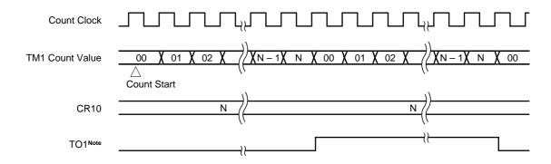
Note Initial value of TO1 output can be set at bits 2 and 3 (LVS1 and LVR1) of the 8-bit timer output control register (TOC1).
