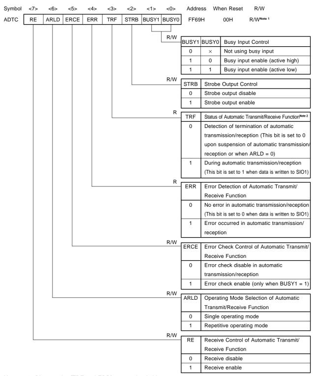
Figure 17-4. Automatic Data Transmit/Receive Control Register Format
