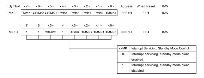
Note WTMK flag controls standby mode clear enabled/disabled. The interrupt function does not control.
