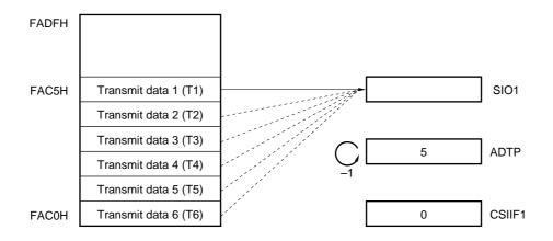
Figure 17-12. Buffer RAM Operation in 6-Byte Transmission (in Basic Transmit Mode) (2/2)
