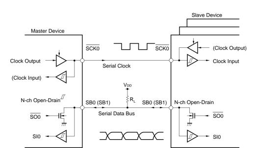
Figure 16-28. Pin Configuration
