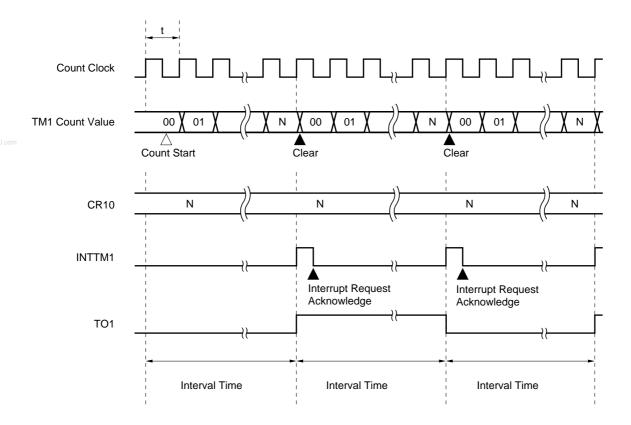
Figure 9-8. Interval Timer Operation Timings
