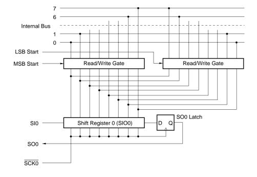
Figure 15-10. Circuit of Switching in Transfer Bit Order
