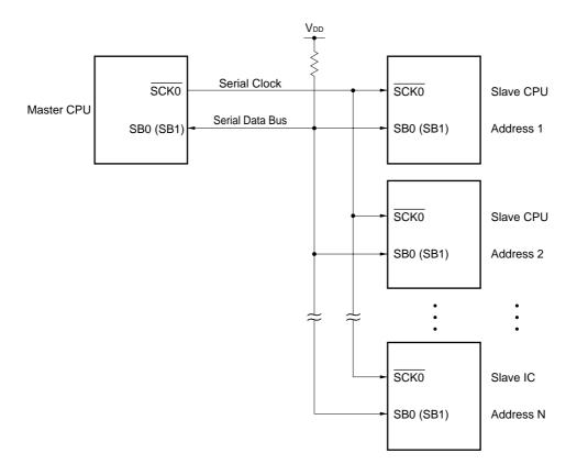
Figure 15-11. Example of Serial Bus Configuration with SBI
