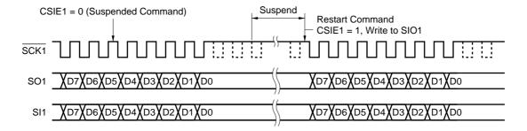
CSIE1: Bit 7 of the serial operating mode register 1 (CSIM1)
