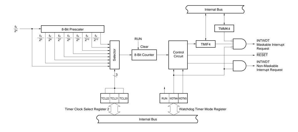
Figure 11-1. Watchdog Timer Block Diagram
