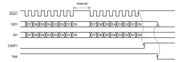
Cautions 1. Because, in the basic transmit/receive mode, the automatic transmit/receive function writes/reads data to/from the buffer RAM after 1-byte transmission/reception, an interval is inserted until the next transmission/reception.
