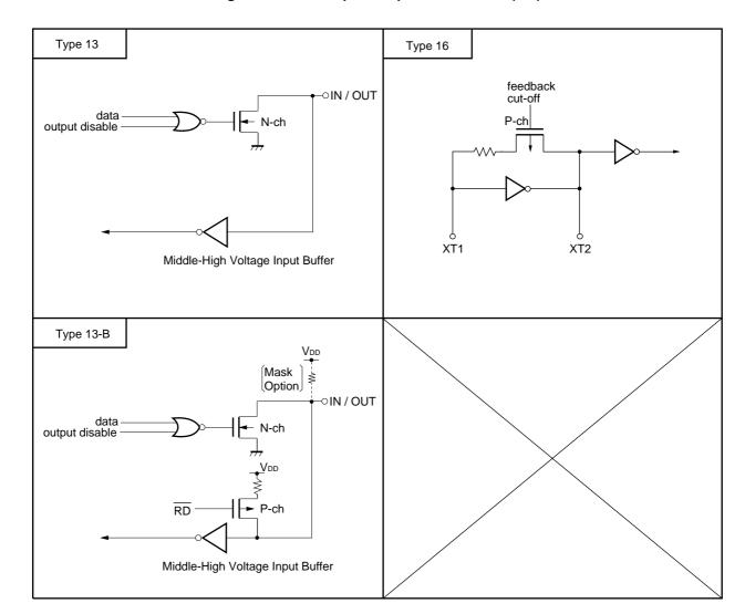
Figure 3-1. Pin Input/Output Circuit List (2/2)
