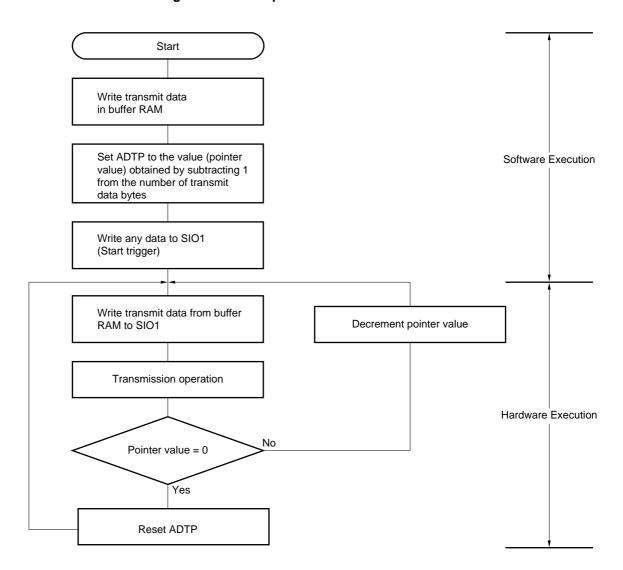
Figure 17-14. Repeat Transmit Mode Flowchart
