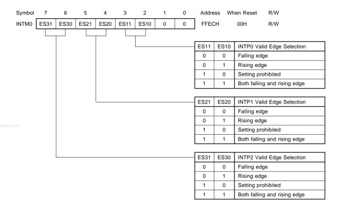
Caution To specify the INTP0/P00/TI0 pin valid edge, bit 1 to bit 3 (TMC01 to TMC03) of the 16-bit timer mode control register (TMC0) must be set to 0, 0, 0, respectively after timer operation is stopped.
