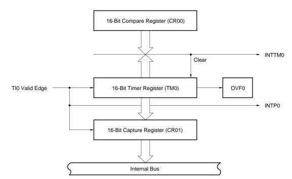
Figure 8-17. External Event Counter Configuration Diagram
