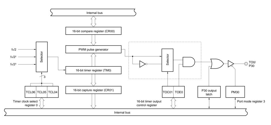
Figure 8-2. 16-Bit Timer/Event Counter (PWM Mode) Block Diagram
