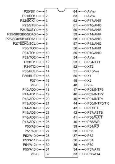
Cautions 1. Connect IC (Internally Connected) pin directly to Vss.
