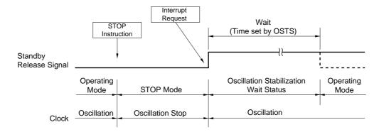
**Remark** The broken line indicates the case when the interrupt request which has cleared the standby status is acknowledged.
