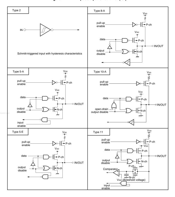
Figure 4-1. Pin Input/Output Circuit List (1/2)
