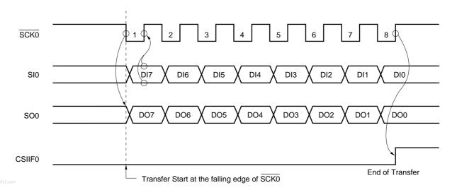
Figure 16-9. 3-Wire Serial I/O Mode Timings
