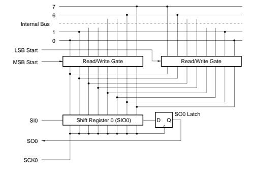
Figure 16-11. Circuit of Switching in Transfer Bit Order
