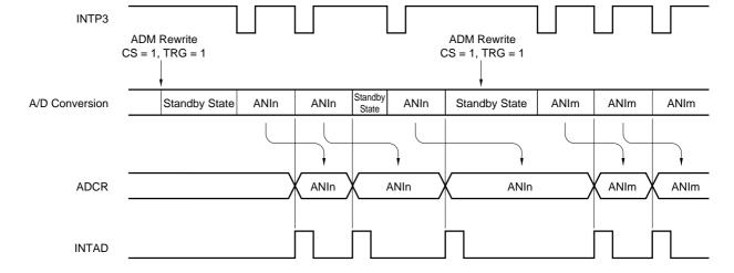
Figure 14-6. A/D Conversion by Hardware Start
