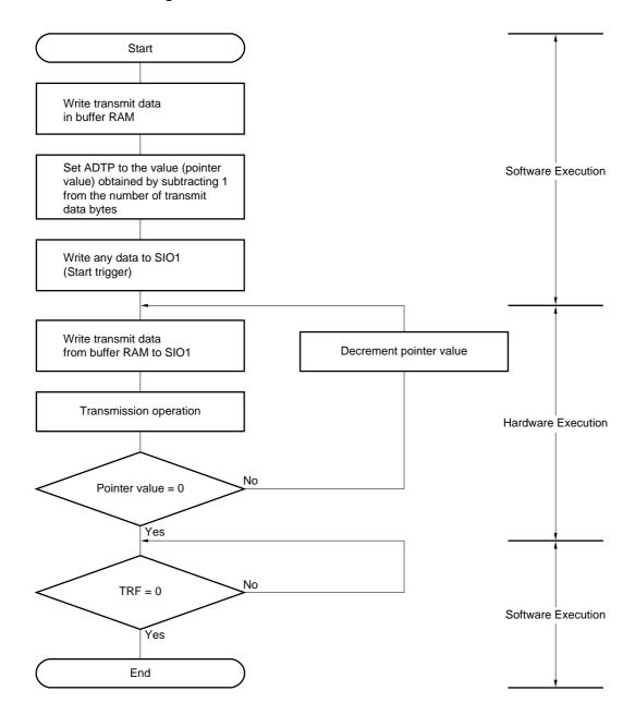
Figure 17-11. Basic Transmit Mode Flowchart
