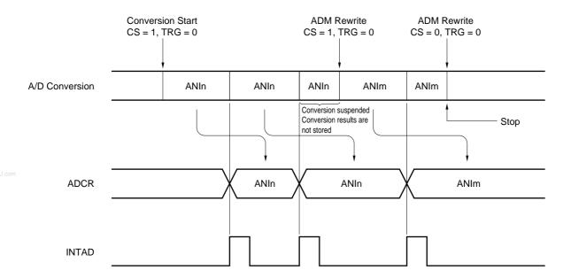
Figure 14-7. A/D Conversion by Software Start
