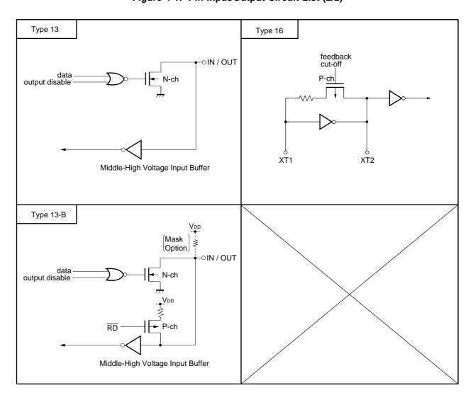
Figure 4-1. Pin Input/Output Circuit List (2/2)
